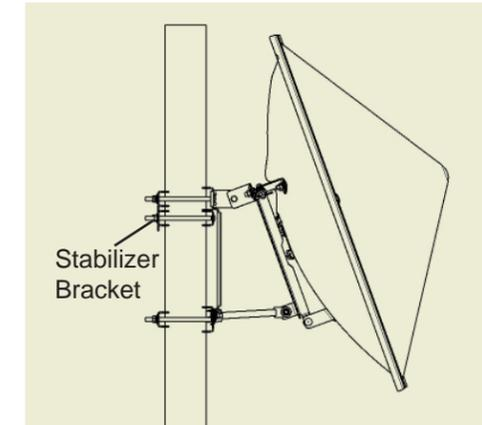
Elevation adjustment bar is on bottom of antenna and stabilizer bracket is set below top bracket of parabolic mount.
