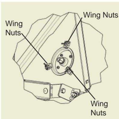
Adjust feed polarization if required. Feed is attached and set for vertical polarization when antenna is mounted on a vertical pipe. To change polarization, loosen 3 wing nuts - rotate feed 90°, then tighten wing nuts. This operation may be performed at any time during installation through final alignment.
