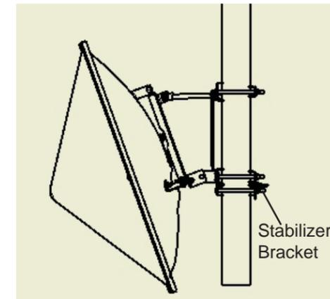
Elevation adjustment bar is on top and stabilizer bracket is on the bottom.
