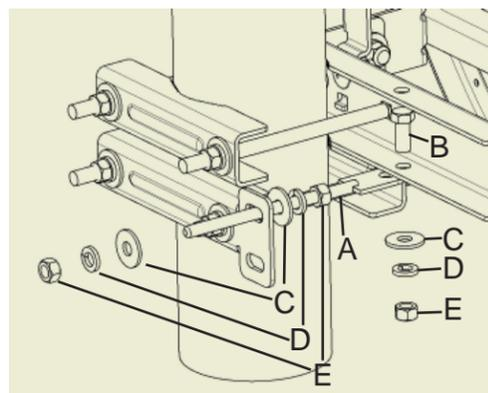
When alignment is completed tighten all hardware.
